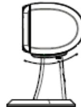
Step 8: Slide the Voice2 loudspeaker in the cradle to adjust the tilt. When the loudspeaker has been appropriately positioned, firmly hand-tighten the tilt adjustment knobs to lock the loudspeaker in place. Do NOT over-tighten.
