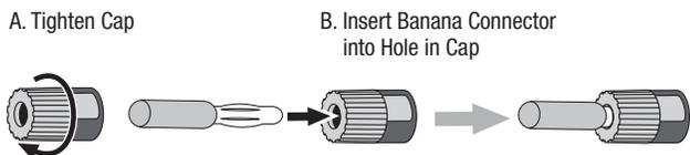
Always connect the colored (+) terminal on the AVR to the (+) terminal on the speaker (usually red), and the black (-) terminal on the AVR to the (-) terminal on the speaker (usually black).
