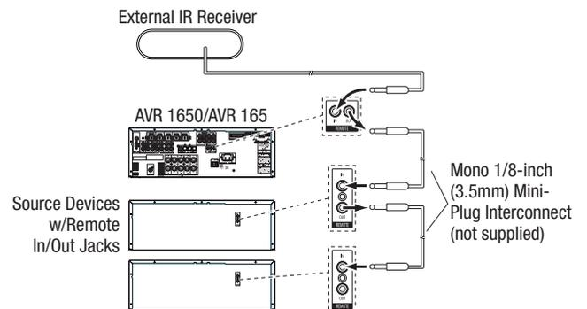
To control more than one source device through the AVR's IR Remote Out connector, connect all sources in "daisy chain" fashion, connecting each device's IR output connector to the next device's IR input connector, starting with the AVR.
