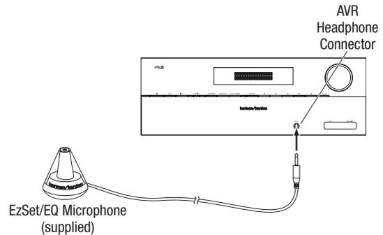
2. Place the microphone at ear height in your listening position. The microphone features a threaded insert on the bottom for mounting on a camera tripod.
